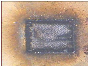
165W average, 800W peak, 5KHz 165µsec on time and 80mg remove, much shaper defined edges compare to CW
