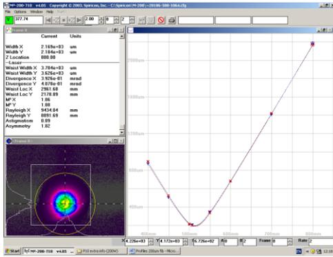
**Fig. 3:** Beam profile of a 400W SM laser
