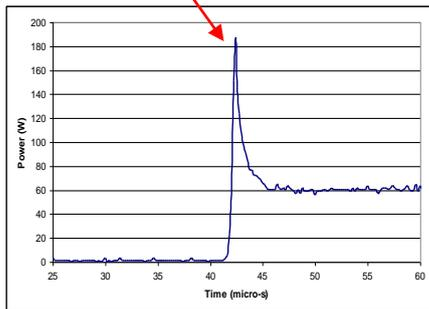
Initial pulse spike expanded view duration around 1 microsecond
