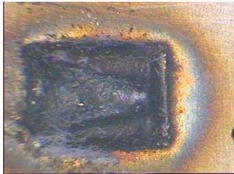
200W, CW, 26 seconds, 50 passes, and 10mg removed.
