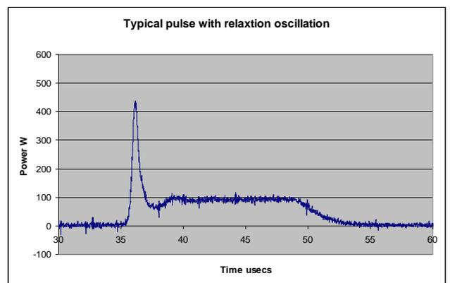
**Fig.5:** Typical output waveform with relaxation pulse
