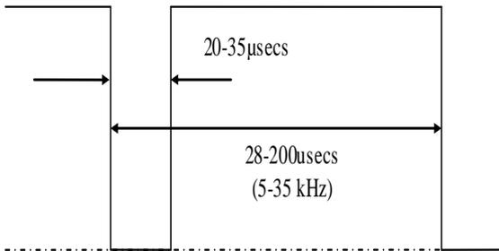
**Fig.4:** Turning the laser off produces a relaxation pulse typically X4-5 the CW level.
