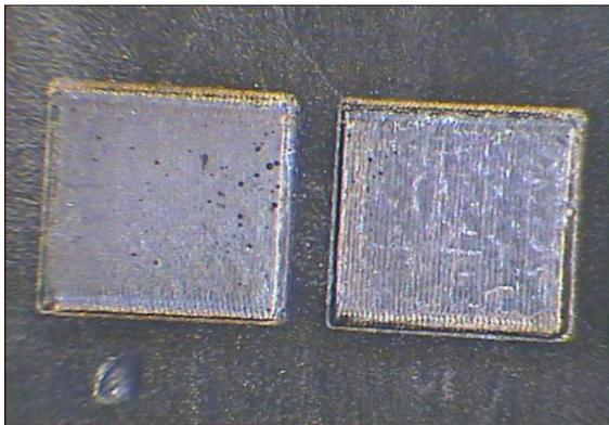
**Fig. 12:** 3mm HastalloyX alloy, 20 passes (left image) and 40 passes (right image), 15 kHz, 800W peak
