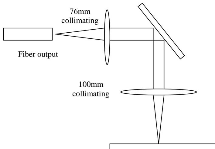
**Fig. 8:** Optical set up for ablation
