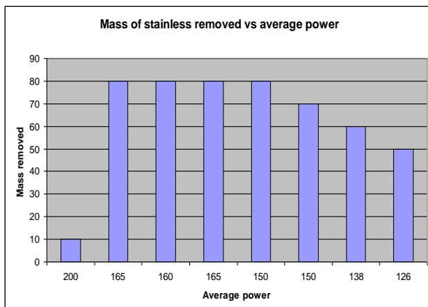
**Fig.9:** Mass removed in 2mm stainless steel
