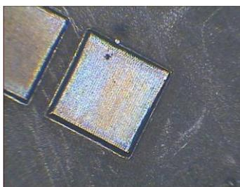
165W average, 800W peak, 15KHz 55sec on time and 80mg remove, the photograph doesn't illustrate clearly but this was the best finish with argon shield gas
