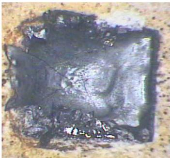
200CW, 26 seconds, very massy with excessive cracking
