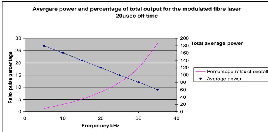
**Fig.7:** Average power and % of total power for the modulated fiber laser 20μsecs off time
