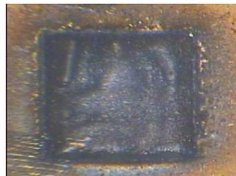
165W average, 800W peak, 15KHz 55µsec on time and 80mg remove, the photograph doesn't illustrate clearly but this was the best finish with the assist gas
