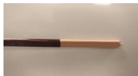
**Figure 4.** Hairpin ablation of dielectric coating prior to welding using ns pulsed fiber lasers offers a cleaner, faster and more repeatable result that wire brush mechanical removal.
