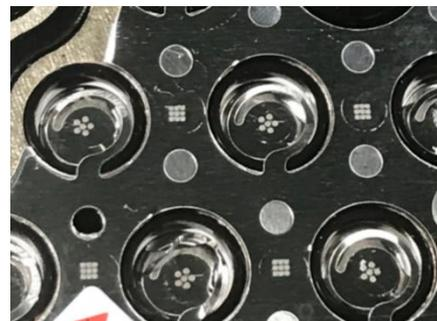
**Figure 2.** Battery tab welding using nanosecond laser welding achieves high strength and electrical conductivity without overpenetration. Thin metals and contained electrolytes under pressure make this a demanding application.
