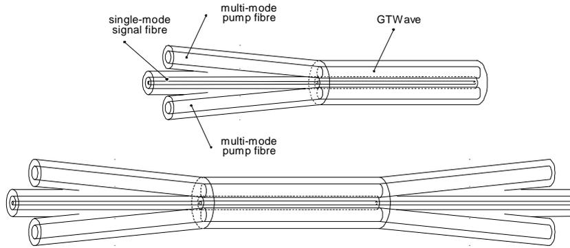
Figure 3. (Top) GTWave™ fiber is 'broken-out' into two multi-mode pump fibers and a single-mode signal fiber for ease of launching pump and signal light
