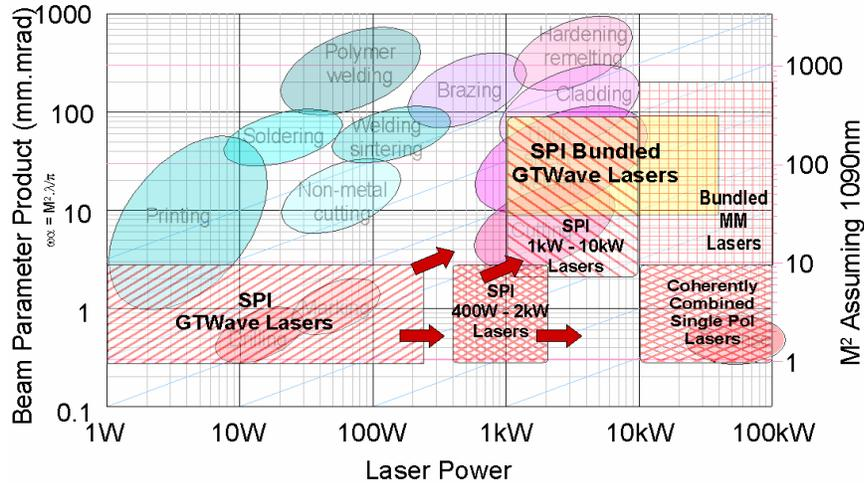
Figure 13: Application Space for Fiber Lasers
