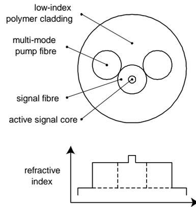
Figure 2. Cross-section and refractive index profile of GTWave™
