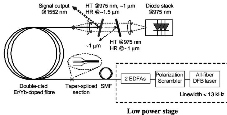
Figure 12: 1552 nm single-frequency MOPA configuration
