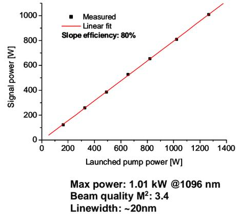
Figure 11: 1kW HPFL with  $M^2 = 3.4$ : August '03
