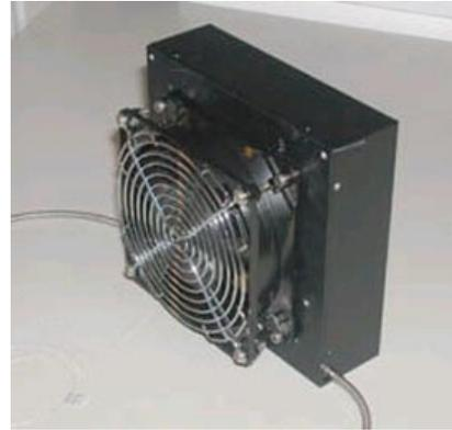
Figure 6: GTWave Laser Cavity Module containing active fiber, Fiber Bragg Grating reflectors and air-cooling heat exchanger
