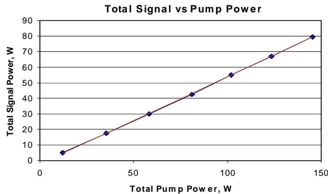
Figure 4: Single GTWave spool performance when pumped at 915nm
