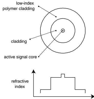
Figure 1. Cross-section and refractive index profile of a standard double-clad fiber
