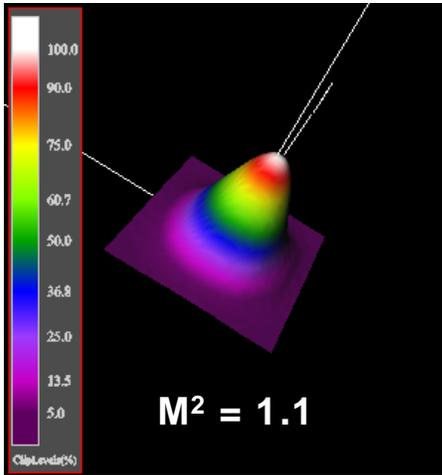
Figure 5: Beam Quality parameter for 100W GTWave concatenated spool lasing at 1085nm
