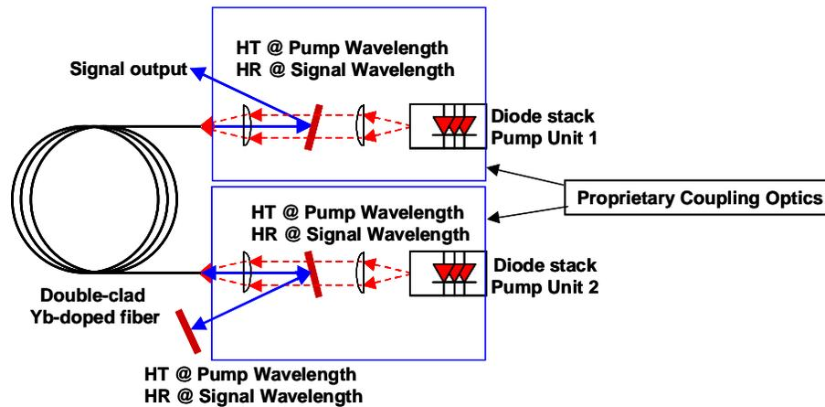
Figure 9: VHPFL: Schematic of dual-ended cladding pumped fiber laser
