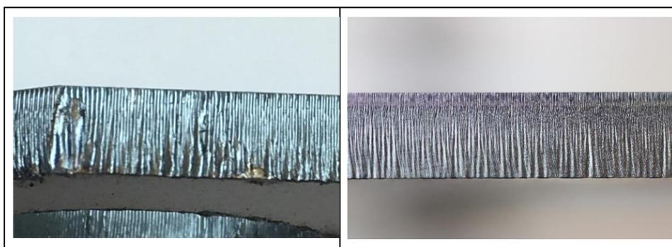
**Figure 4:** 6mm mild steel cutting with (left) 500W SM laser and (right) 500W MM (50µm) laser. Note the strong striations, rough cut-edge and the droplets of dross of the SM laser cut
