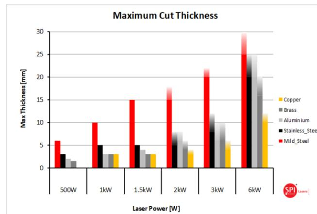
Figure 12: Maximum cutting thickness for laser powers up to 6kW
