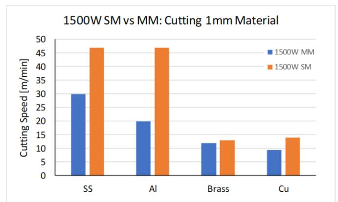
**Figure 9:** Comparison of 1mm cutting for 1.5kW SM and MM lasers
