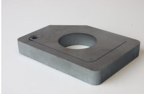
**Figure 7:** 10mm MS cut with 1kW MM laser at 0.6m/min
