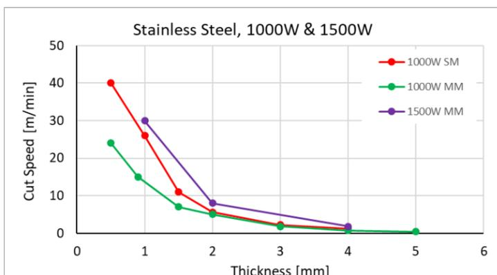
**Figure 10:** 1000W vs 1500W cutting stainless steel
