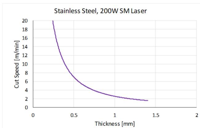
**Figure 2:** Cutting performance of a 200W SM Laser using a 60µm focal spot size
