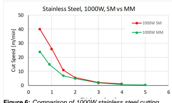
**Figure 6:** Comparison of 1000W stainless steel cutting performance of SM vs MM
