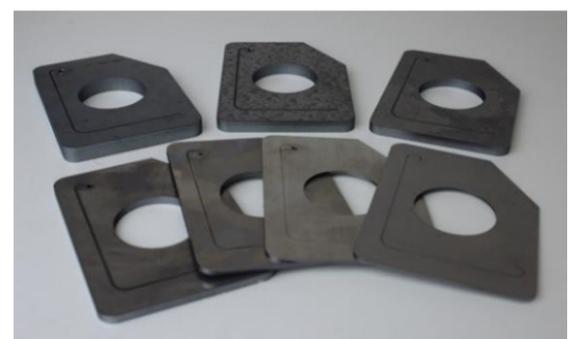
**Figure 5:** Mild steel cutting with 500W MM laser
