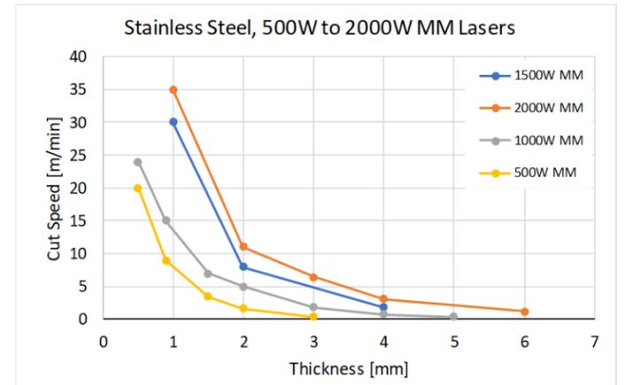
Figure 11: 500W vs 2000W cutting stainless steel
