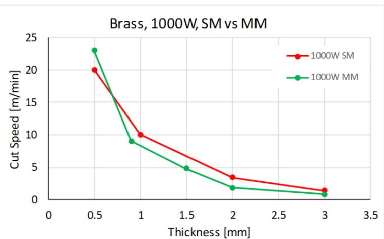
**Figure 8:** Comparison of cut performance for aluminium and brass for 1kW SM and MM
