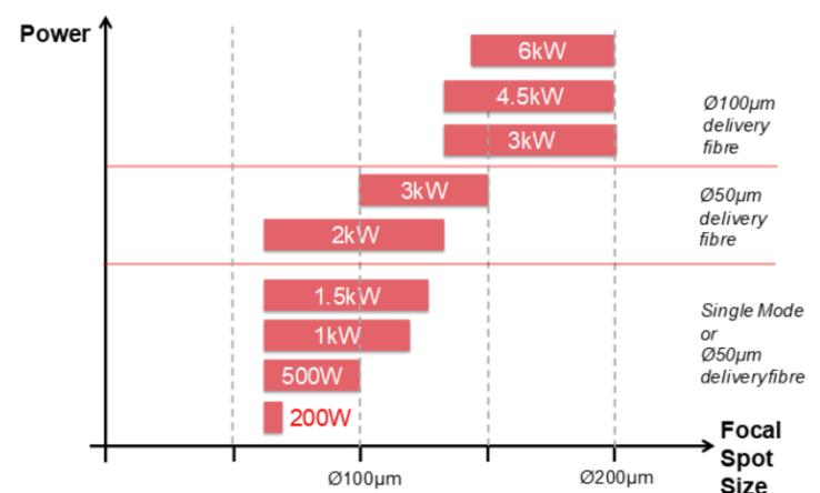
**Figure 1:** Typical range of focal spot sizes used for cutting within the laser power range 200W to 6kW
