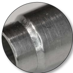
Welding 304 stainless steel
